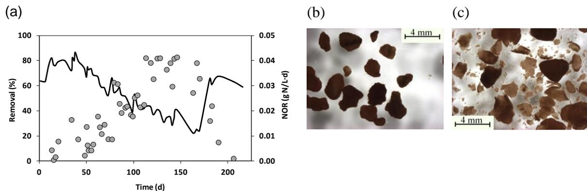
**Figure 1.1** Profile of nitrogen removal percentage (—) and nitrite oxidizing rate (NOR) (●) in the lab scale SBR(a). And images of the granules (zoom: 6.5x). (b) Inoculum and (c) on day 120.
